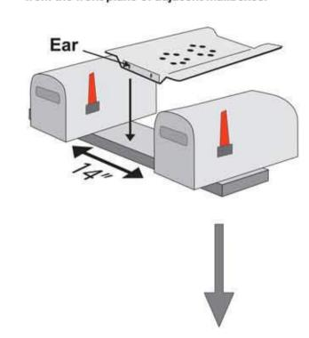
Attach the mounting plate to the post using the four machine bolts that came with the post. A drive socket, wrench or crescent wrench may be used to tighten and secure the bolts to the Fast-Trak® mounting plate.
