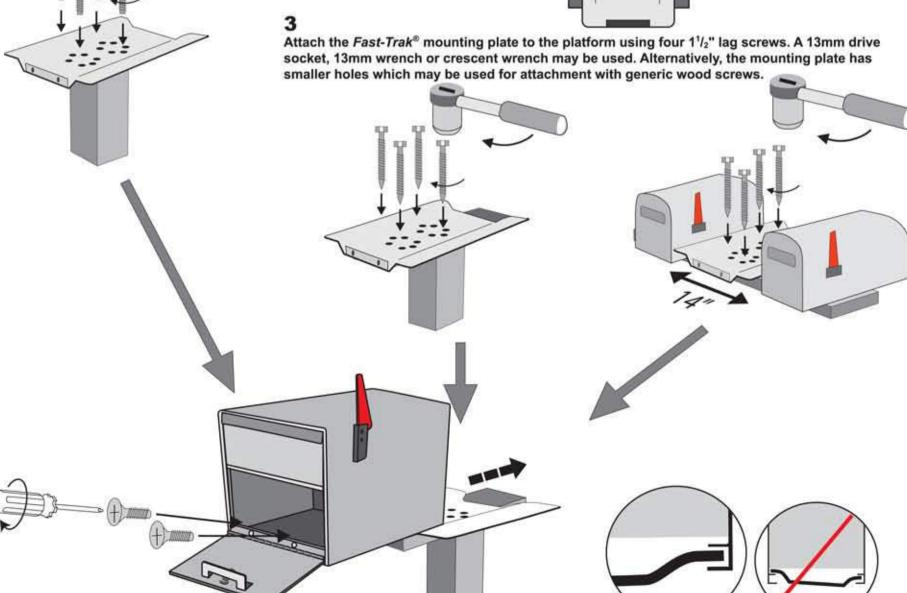
Simply slide MAIL BOSS® onto FAST-TRAK® mounting plate and secure with two machine screws provided.
